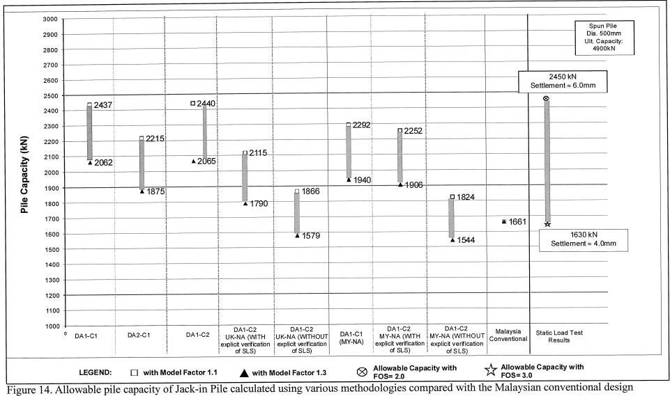
method and static pile load test results (\$500mm Spun Pile – Site D).
