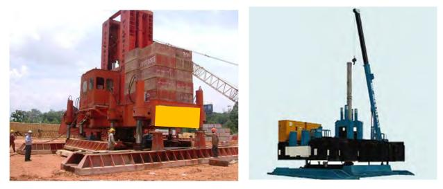
Figure 1. Typical high capacity jack-in pile machine in Malaysia.
