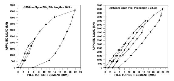
Figure 12. Load-settlement results of pile load test at Site D.
