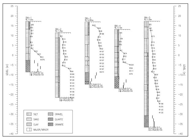
Figure 8. Borehole profiles at Site D.
