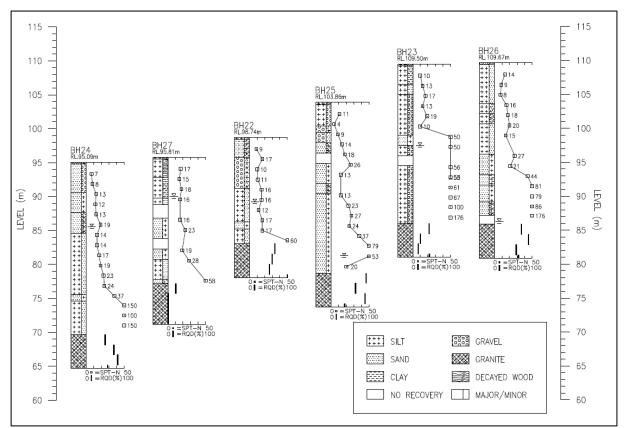
Figure 6. Borehole profiles at Site B.
