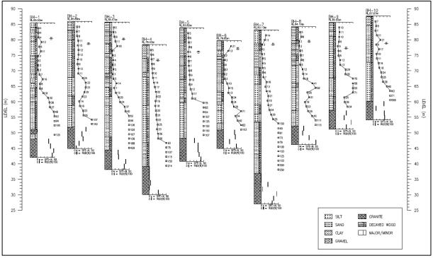
Figure 7. Borehole profiles at Site C.
