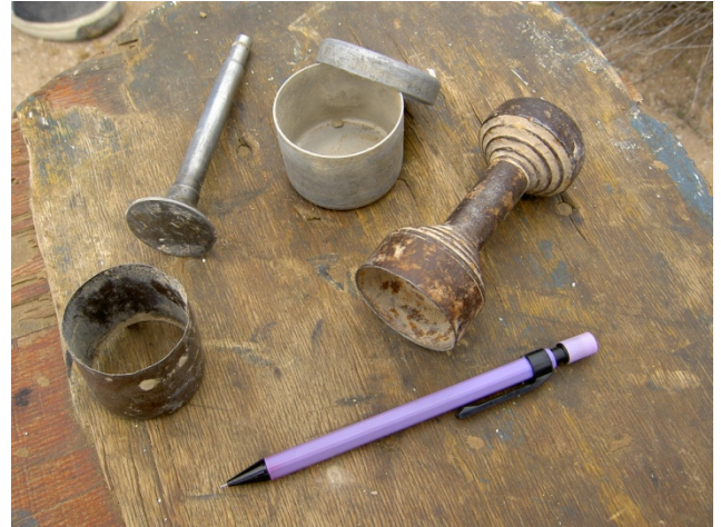
Figure 25. Tools for Collection of Soil Samples.
