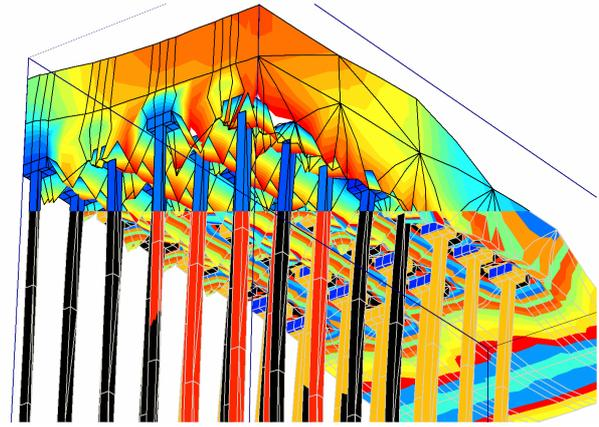
Fig. 8 Results of 3D FEM analyses showing 'mushroom' problems (bottom view).
