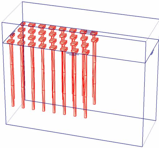
Fig. 6 Typical 3D FEM model of piles and pilecaps.
