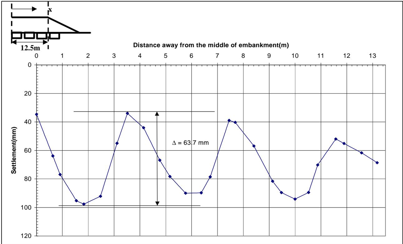
Fig. 9 Settlement profile before remedial treatment across the embankment.
