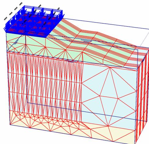
Fig. 5 Typical 3D FEM model of embankment.
