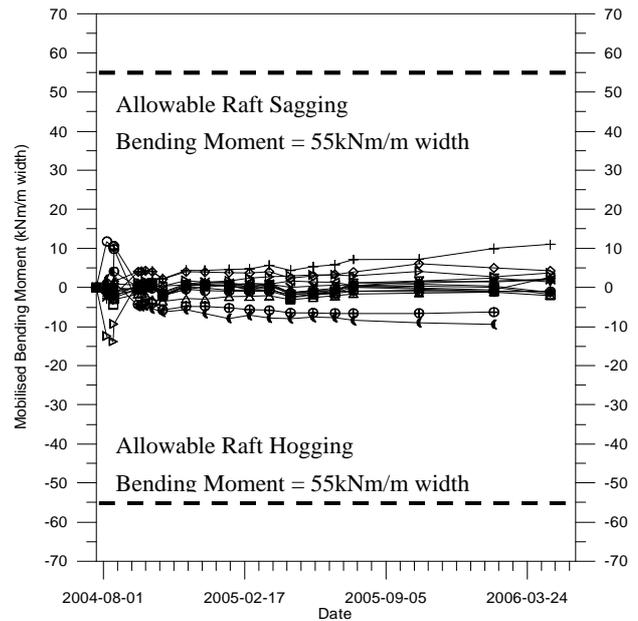
Fig. 20 Interpreted mobilised bending moment
