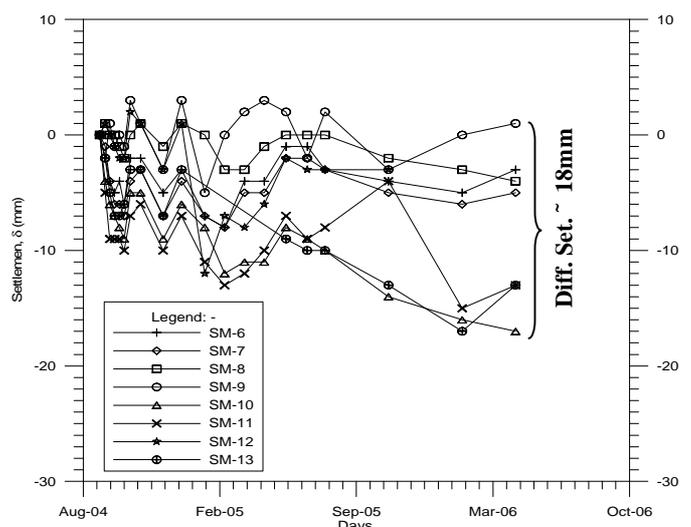
Fig. 18 Settlement markers at untreated bound
