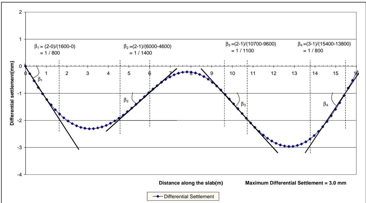
Fig. 10 Settlement profile after remedial treatment across embankment using RC raft at shallow depth
