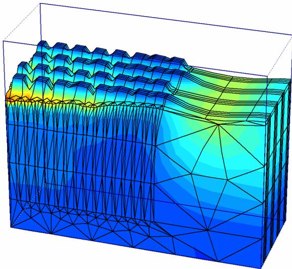
Fig. 7 Results of 3D FEM analyses showing 'mushroom' problems (top view).
