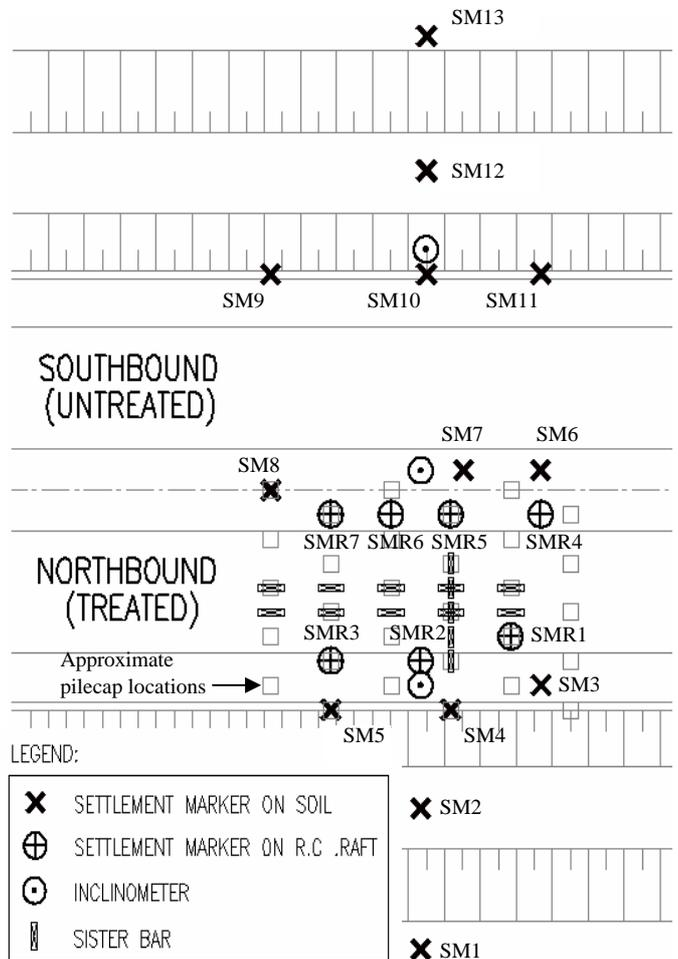
Fig. 17 Layout plan of instrumentation monitoring
