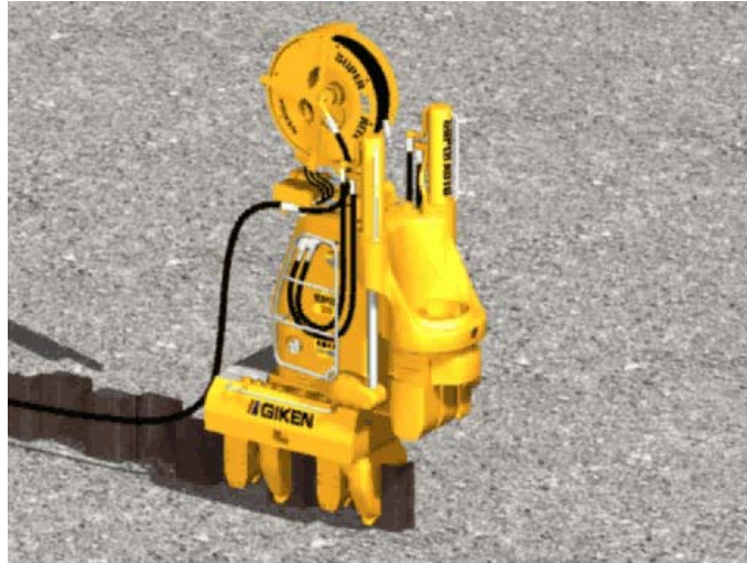
Figure 8: Typical press-in piling system using Japanese technologies.
