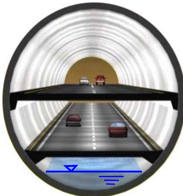
Figure 13: Cross-section of SMART Tunnel ( www.smarttunnel.com.my )
