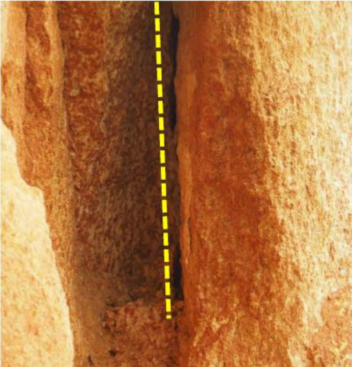
Photo 6: Decomposed feldspar and mica infilling in the relict joint
