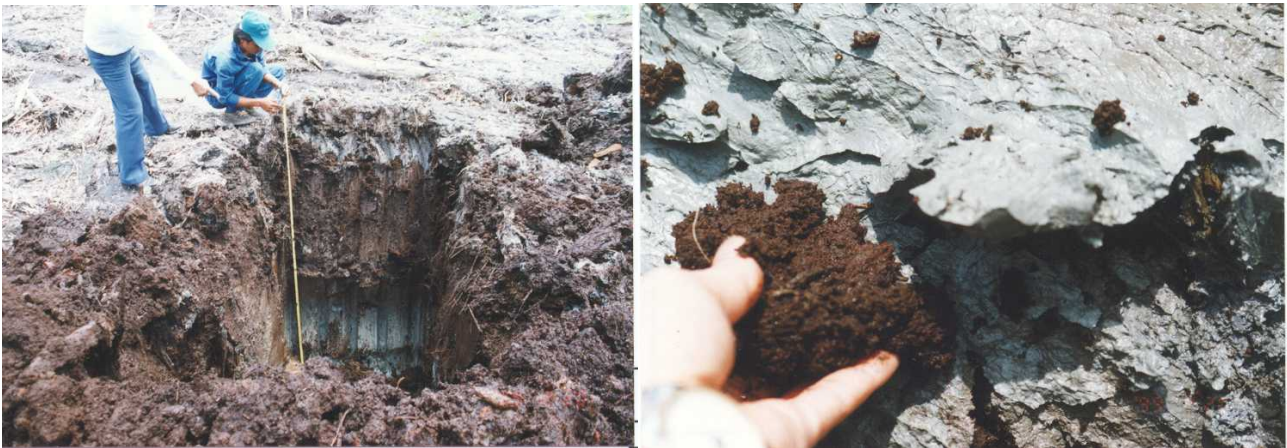
Plate 6: 1.5 to 3m thick clean amorphous peats overlying soft compressible marine clay deposits
