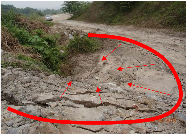
Plate 10: Sinkhole developed in overburden behind the quarry benches
