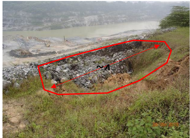
Plate 10: Sinkhole developed in overburden behind the quarry benches
