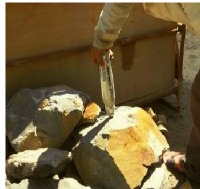
Figure 4 Rebound Hammer Test
