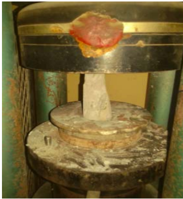
Figure 2 Unconfined Compression Strength Test
