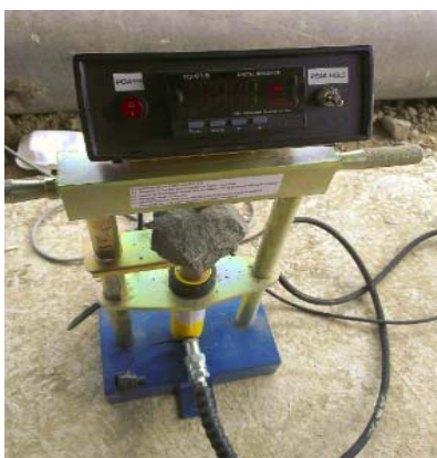
Figure 3 Point Load Test
