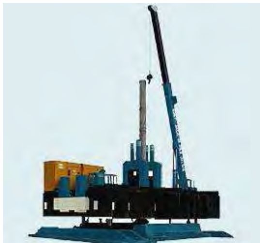
Figure 1: Typical high capacity jack-in pile machine in Malaysia.
