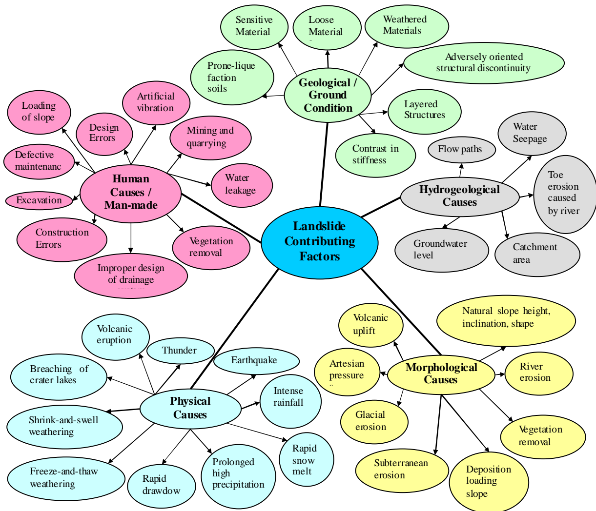
Fig.4 Landslide Contributing Factors
