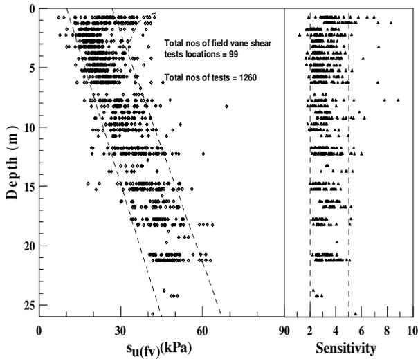
Fig. 2. Undrained shear strength and sensitivity of Klang Clay (from Tan *et al.*, 2004).
