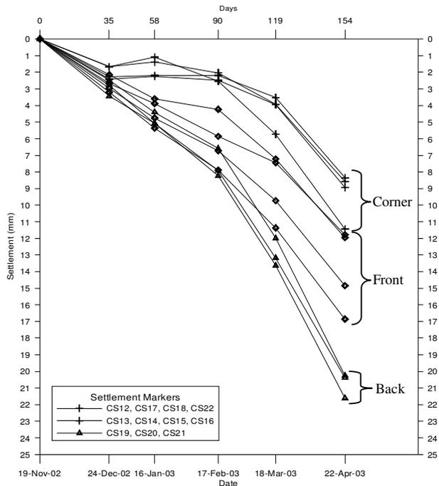
Fig. 12. Settlement monitoring results for Block 3.
