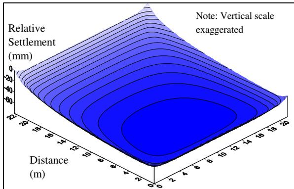
Fig. 7. Settlement profile for semi-detached house (intermediate unit).
