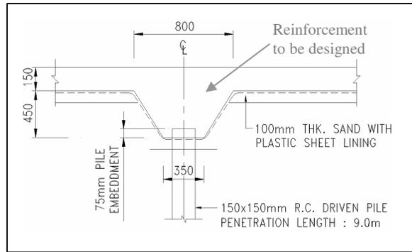
Fig. 9. Typical cross-section of strip raft foundation system.
