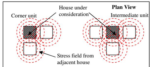
Fig. 4. Effect of adjacent houses on settlement (semi-detached house).
