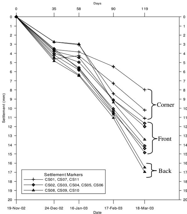
Fig. 11. Settlement monitoring results for Block 2.
