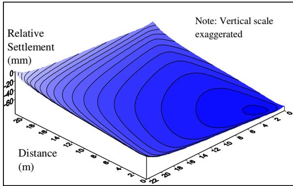
Fig. 6. Settlement profile for semi-detached house (corner unit).
