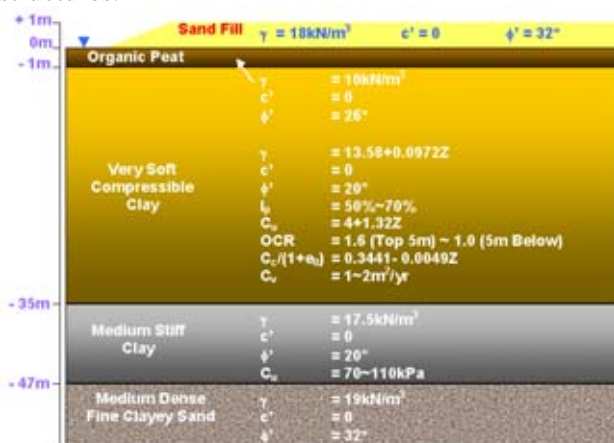
Figure 2 Subsoil Condition of Project Site
