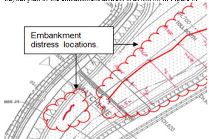
Figure 3 Layout Plan of embankment distress
