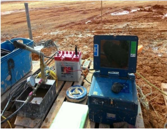
Figure 2: Crosshole Seismic Testing
