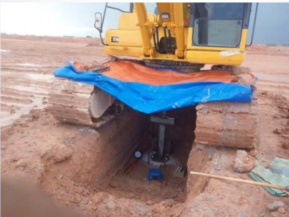
Figure 4: Plate Bearing Test
