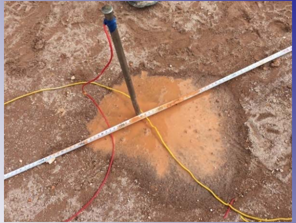
Figure 3: Earth Resistivity Test (Wenner Array)
