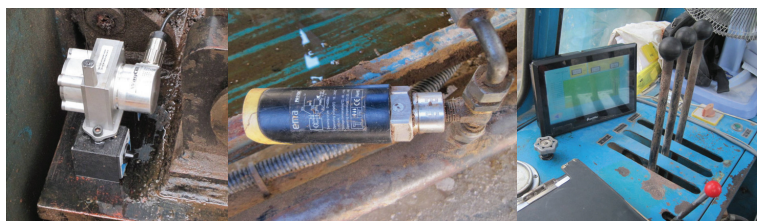
Figure 4. Photo showing wire spring LVDT penetration decoder mounted magnetically onto the jacking frame, pressure transducer to measure jacking pressure and LCD panel placed inside the operator cabin for immediate feedback on monitoring results.
