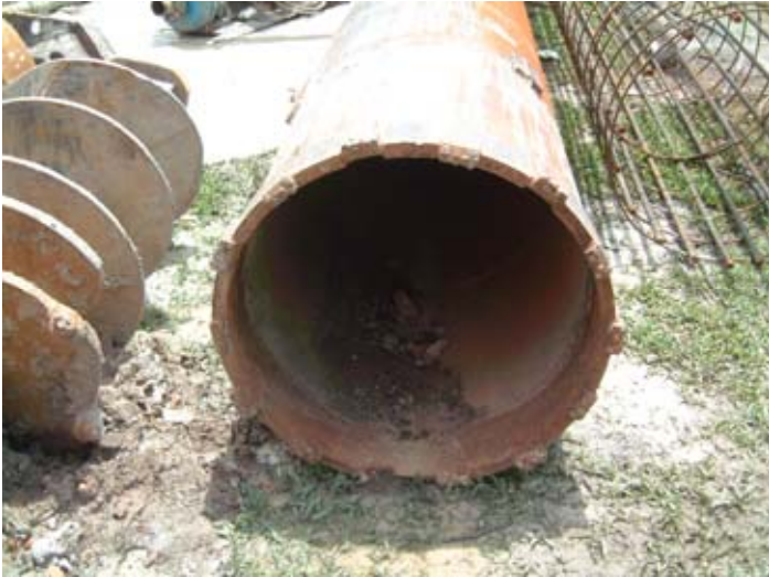
Figure 20: Modified rock coring tool for bored pile construction in limestone areas.
