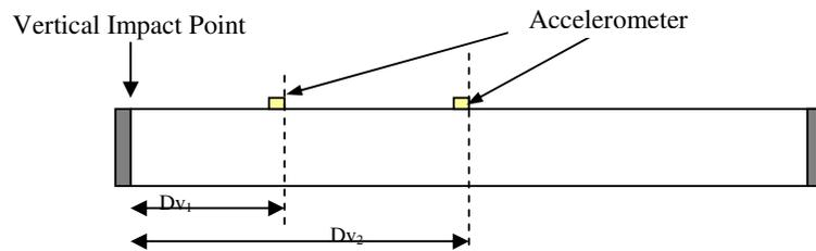
Figure 2: Measurement of vertical velocity
