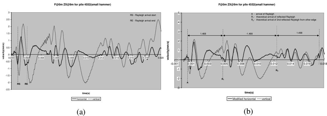
Figure 5: Velocity response of pile 4552 (a) before (b) after correction factor is applied
