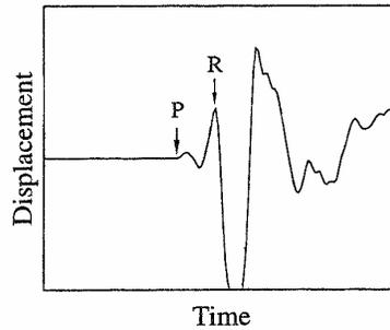
Figure 3: Displacement signal for test performed at distance 0.15 m (Sansalone, Lin et al.,1997)
