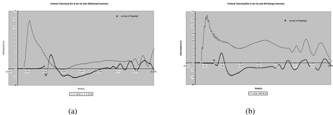
Figure 4: Identification of arrival of incident Rayleigh waves in (a) pile 4552 (b) pile 8474
