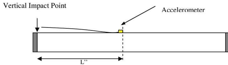
Figure 1: Measurement of simultaneous horizontal-vertical velocities
