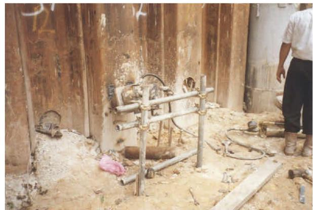
Figure 3 : View of the Pull-Out Test Arrangement
