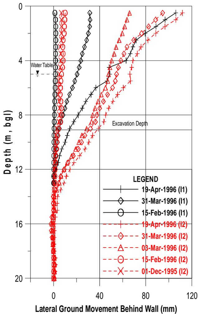
Figure 7 : Lateral Ground Movements Behind Wall
