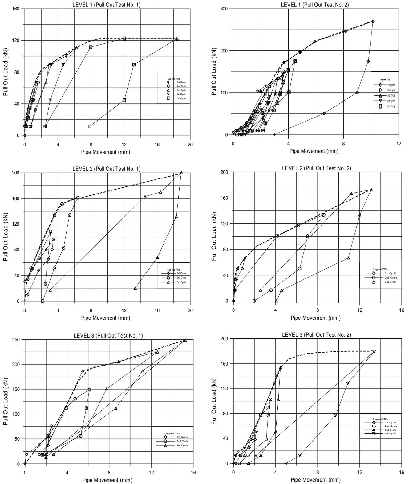
Figure 6 : Pull-Out Tests for 3 Levels of Jack-In-Pipe Anchor
